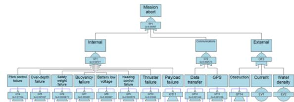
Figure 1. High-level fault tree model for BRIDGES glider mission abort.
