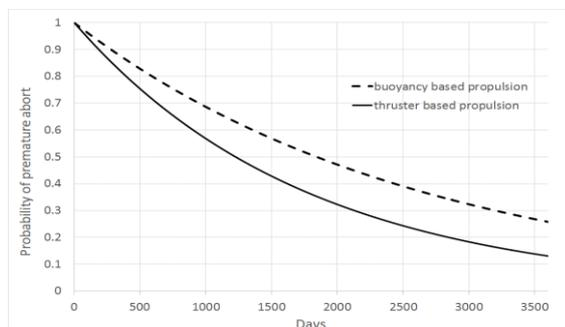
Figure 2. Reliability profile for the BRIDGES glider considering buoyancy-based propulsion and thruster-based propulsion.
